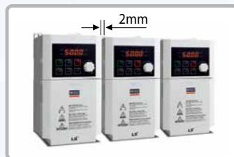
Side-by-side Installation (2mm between drives)
