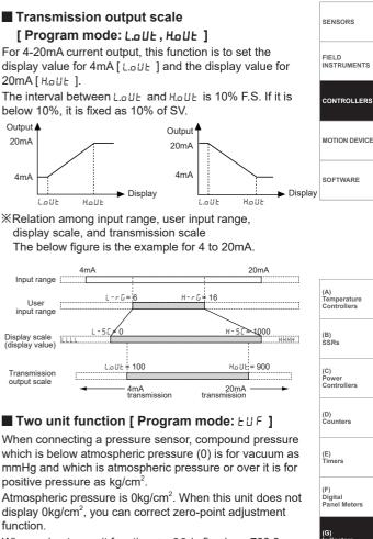
When using two unit function, L - 5L is fixed as -760.0 L - 5L parameter is displayed but you cannot set this. You can set H - 5L within 0 to 19999 range.
