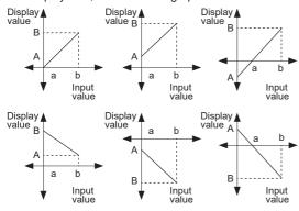
Display scale function is able to change display value for max./min. measured input by setting high limit scale [H - 5L] and low limit scale [L - 5L] in program mode. %E.g.) Set high/low scale value (input range is 0 to 10V)
