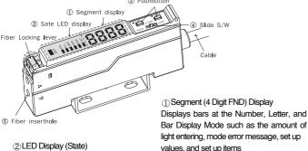
Displays the state of Fiber Sensor
